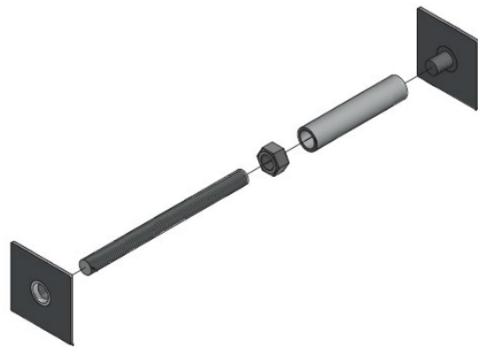
Diagram 8 - Typical compression spreader detail
